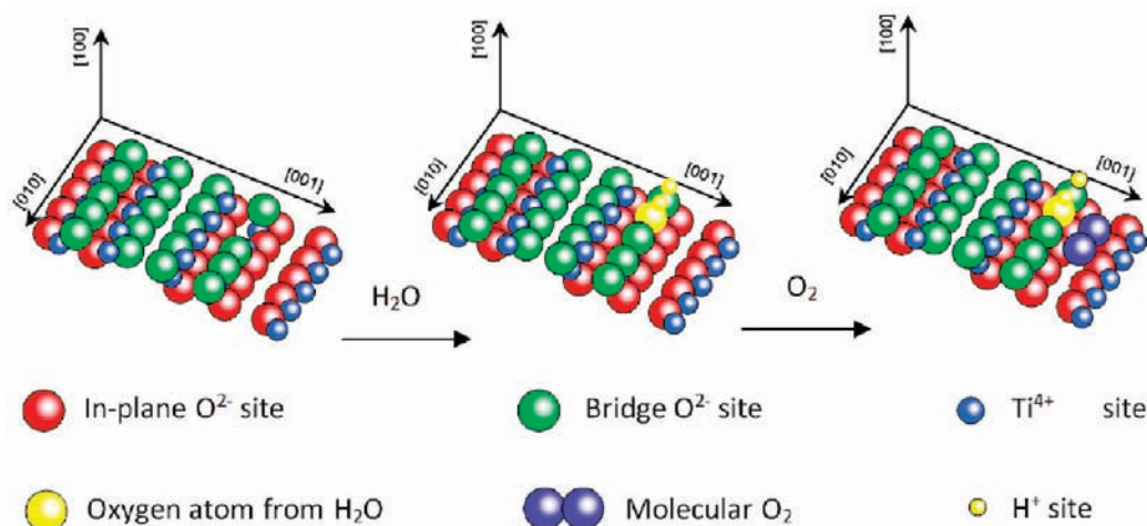
Figure 7. Proposed \text{H}_2\text{O} and \text{O}_2 adsorption process on exposure to the (100) plane in anatase.
